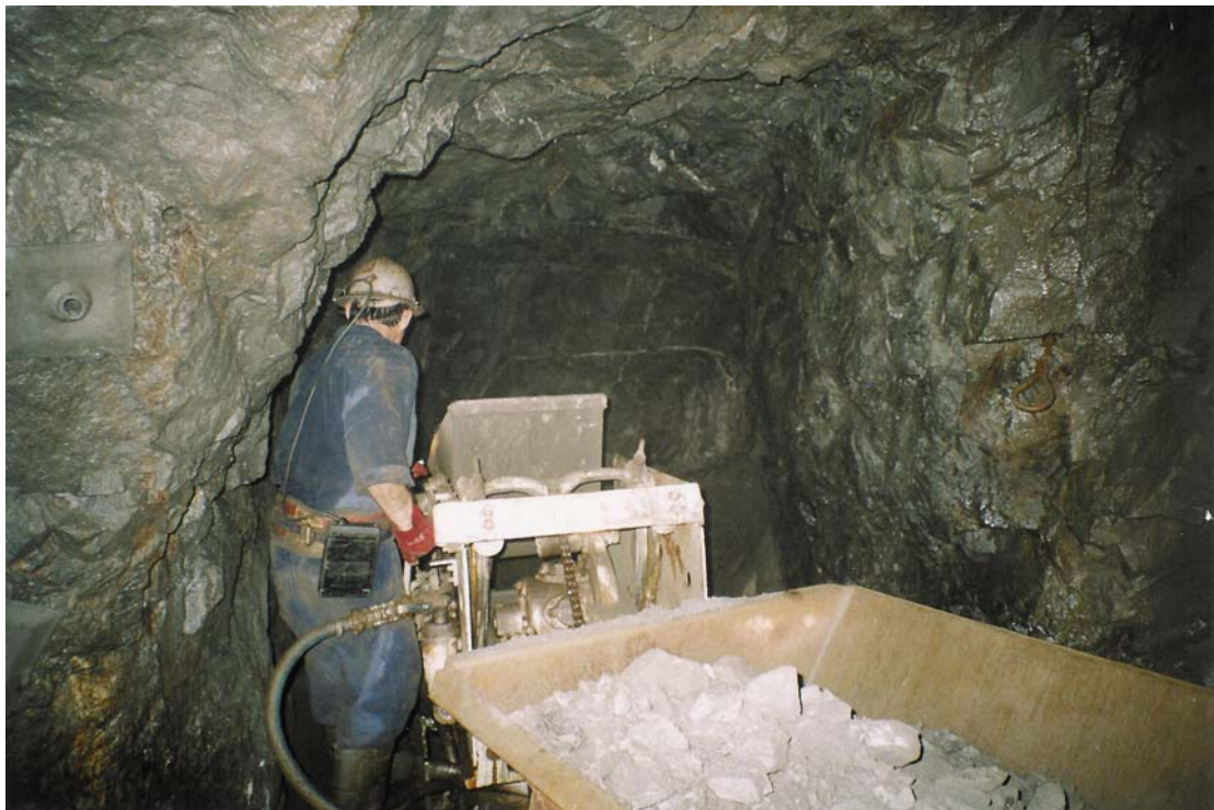
Bogging in 2 Level South Drive, Sand Queen Mine Main Shaft, Comet Vale.
